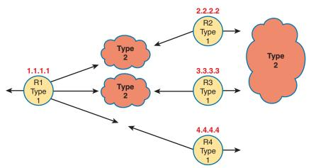
Figure 21-17 Type 1 and Type 2 LSAs in Area 0, Assuming a Single-Area Design
