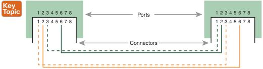
Figure 2-11 Crossover Ethernet Cable Pinouts
