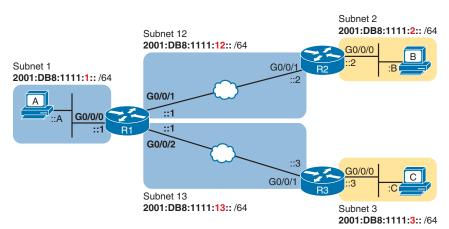
Figure 28-2 Sample Network with IPv6 Addresses
