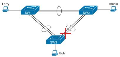
Figure 9-12 Two-Segment EtherChannels Between Switches
