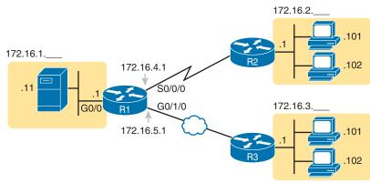
Figure 16-6 IPv4 Addresses Used in Example 16-2
