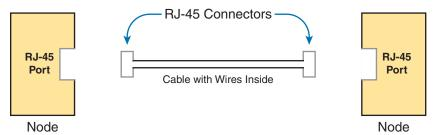
Figure 2-6 Basic Components of an Ethernet Link
