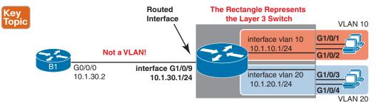
Figure 18-5 Routing on a Routed Interface on a Switch
