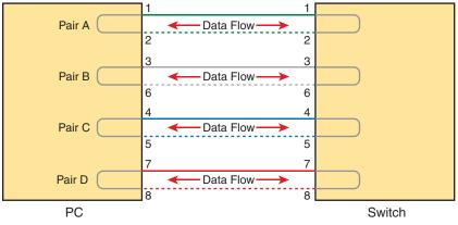
Figure 2-13 Four-Pair Straight-Through Cable to 1000BASE-T
