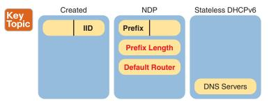
Figure 28-9 Sources of Specific IPv6 Settings When Using SLAAC
