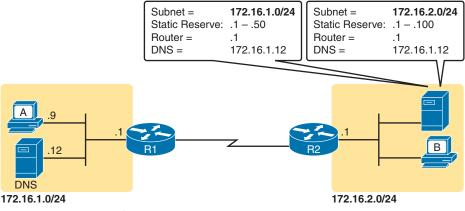
Figure 19-4 Preconfiguration on a DHCP Server
