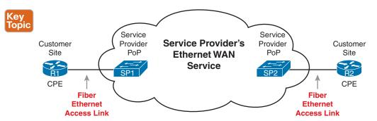
Figure 3-7 Fiber Ethernet Link to Connect a CPE Router to a Service Provider's WAN
