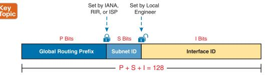
Figure 26-6 Structure of Subnetted IPv6 Global Unicast Addresses
