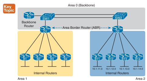
Figure 21-13 Three-Area OSPF with D1 and D2 as ABRs
