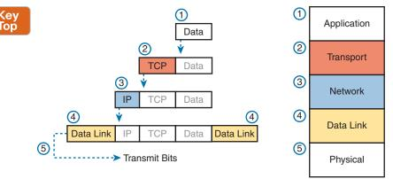
Figure 1-12 Five Steps of Data Encapsulation: TCP/IP
