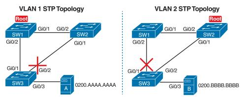
Figure L-4 Two Different STP Topologies for Same Physical LAN, Two Different VLANs
