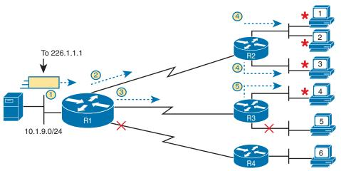
**Figure K-2** *Example of a Multicast Packet Flow for Three Registered Hosts* Following the steps in the figure:
