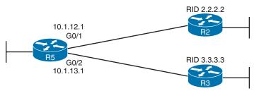
Figure 24-2 Example Network to Demonstrate OSPF Process Shutdown
