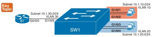
Figure 18-3 Physical Interfaces and Subnets for Layer 3 Switching Example
