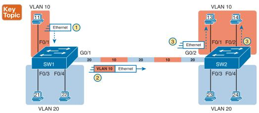
Figure 8-5 VLAN Trunking Between Two Switches
