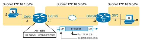
Figure 17-9 Routing Step 4 on Router R1 with a LAN Outgoing Interface
