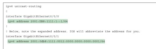
**Example 27-2** Configuring Static IPv6 Addresses on R2
