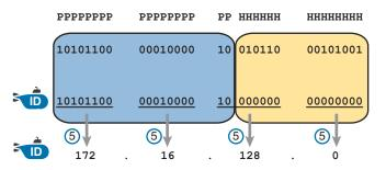
Figure 14-5 Converting the Subnet ID from Binary to DDN
