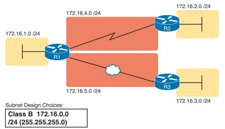
Figure 11-20 Example of Subnets Assigned to Different Locations
