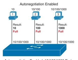
Autonegotiation Enabled, 10/100/1000 Ports **Figure 7-1** *IEEE Autonegotiation Results with Both Nodes Working Correctly*
