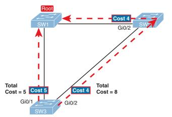
Figure 9-5 How a Human Might Calculate STP/RSTP Cost from SW3 to the Root (SW1)
