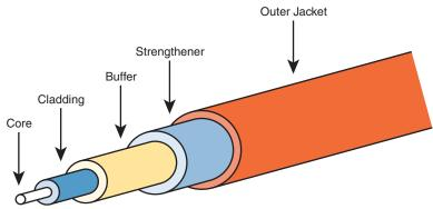
Figure 2-14 Components of a Fiber-Optic Cable
