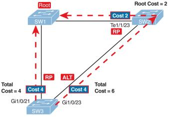
Figure 10-7 Sample Network for Root Switch Election Configuration
