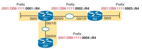
Figure 26-9 Subnets in Company 1, with Global Routing Prefix of 2001:0DB8:1111::/48
