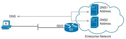
Figure 19-6 Host A Needs to Know the IP Address of the DNS Servers
