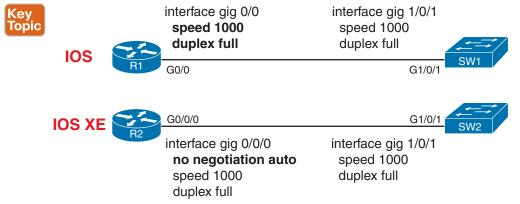
Figure 16-8Router Ethernet Speed, Duplex, and Autonegotiation Configuration
