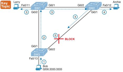
Figure 9-2 What STP/RSTP Does: Blocks a Port to Break the Loop
