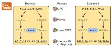
Figure 27-5 Two Partial Examples of the EUI-64 Interface ID Process
