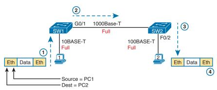
Figure 2-21 Example of Sending Data in a Modern Ethernet LAN
