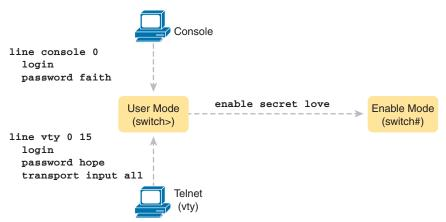
Figure 6-2 Simple Password Security Configuration
