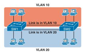
Figure 8-3 Multiswitch VLAN Without VLAN Trunking
