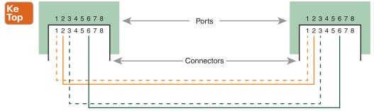
Figure 2-10 10BASE-T and 100BASE-T Straight-Through Cable Pinout
