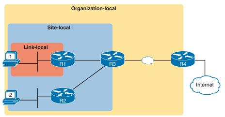
Figure 27-11 IPv6 Multicast Scopes
