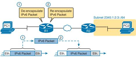
Figure 25-5 IPv6 Router Performing Routine Encapsulation Tasks When Routing IPv6
