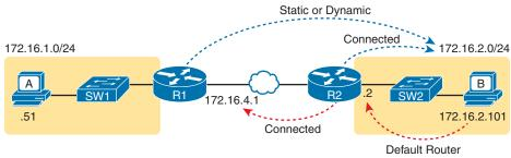
Figure 20-3 Layer 3 Routes Needed for R1's ping 172.16.2.101 to Work
