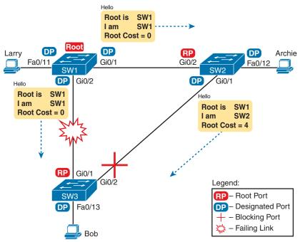
Figure 9-7 Initial STP State Before SW1-SW3 Link Fails
