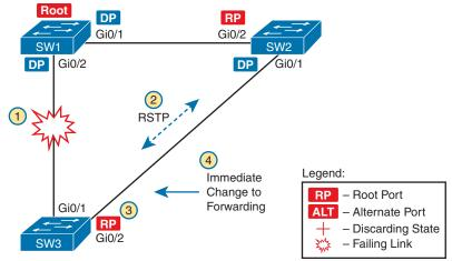
Figure 9-9 Convergence Events with SW3 G0/1 Failure
