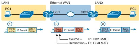
Figure 3-9 Routing over an Ethernet WAN Link
