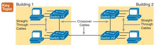
Figure 2-12 Typical Uses for Straight-Through and Crossover Ethernet Cables
