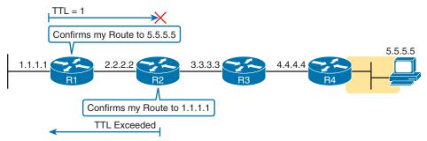
Figure K-7Messages That Cause the traceroute Command to List 2.2.2.2
