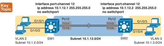
Figure 18-8 Design Used in EtherChannel Configuration Examples
