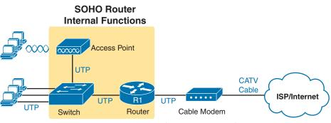
Figure 16-4 Devices in a SOHO Network with High-Speed CATV Internet
