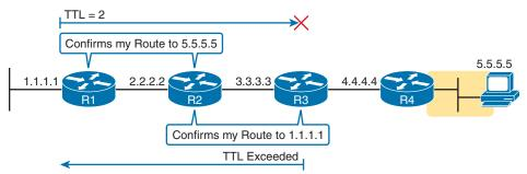
Figure K-8 Messages That Cause the traceroute Command to List 3.3.3.3
