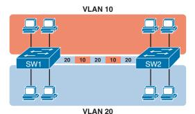
Figure 8-4 Multiswitch VLAN with Trunking
