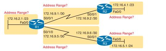
Figure M-4 VLSM Design with Possible Overlap
