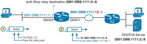
Figure 28-7 DHCPv6 Relay Agent and DHCP IPv6 Addresses
