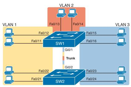
Figure 8-10 Network with Two Switches and Three VLANs
