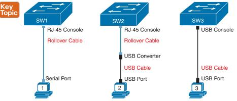
Figure 4-4 Console Connection to a Switch
