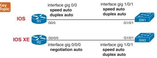
Figure 16-7 Default Ethernet Autonegotiation Configuration: IOS and IOS XE
