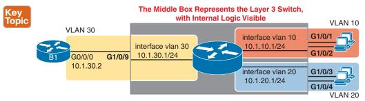
Figure 18-4 Internal VLAN Interfaces for Layer 3 Switching Example
