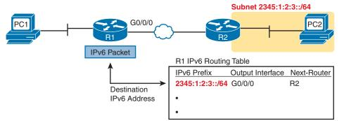
Figure 25-6 Comparing an IPv6 Packet to R1's IPv6 Routing Table
