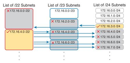
Figure M-3 Selecting Two Subnets Disallows Other Subnets in Different Columns
