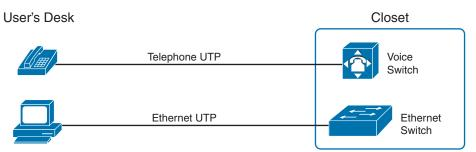
**Figure 8-11** Before IP Telephony: PC and Phone, One Cable Each, Connect to Two Different Devices
