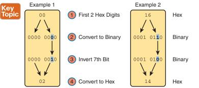
Figure 27-6 Inverting the Seventh Bit of an EUI-64 Interface ID Field
