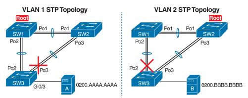
Figure L-5 VLAN Topology with PortChannels Between Switches Example L-4 SW1 and SW2 MAC Tables with PortChannel Ports Listed
