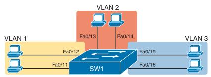
Figure 8-9 Network with One Switch and Three VLANs
