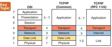
Figure 1-14 OSI Model Compared to the Two TCP/IP Models
