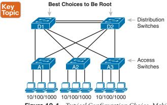
Figure 10-1 Typical Configuration Choice: Making Distribution Switch Be Root
