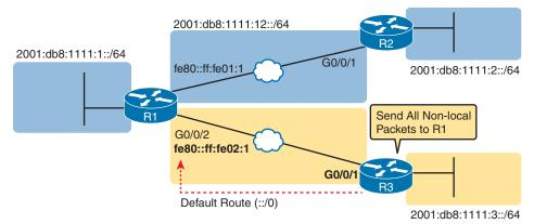
Figure 29-5 Using Static Default Routes at Branch Routers
