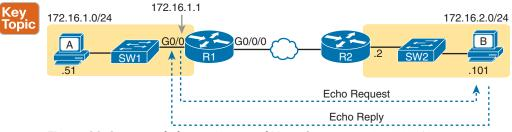
Figure 20-6 Extended Ping Command Tests the Route to 172.16.1.51 (Host A)
