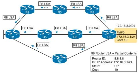
Figure 21-5 Flooding LSAs Using a Link-State Routing Protocol
