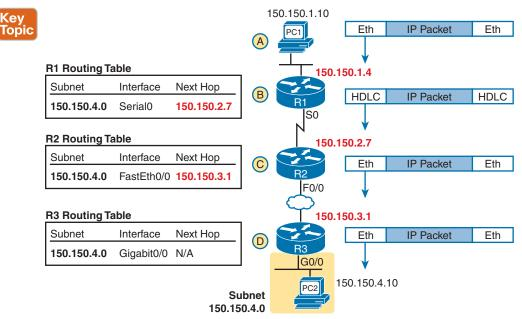
Figure 3-11 Network Layer and Data-Link Layer Encapsulation
