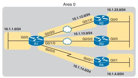
Figure 21-15 Enterprise Network with Six IPv4 Subnets
