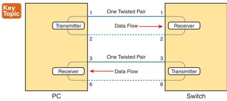
**Figure 2-9** Using One Pair for Each Transmission Direction with 10- and 100-Mbps Ethernet
