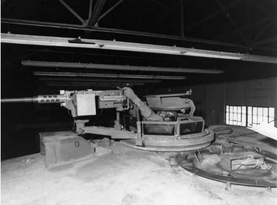
Figure 13.6 Commander difficulty reaching machine gun.
