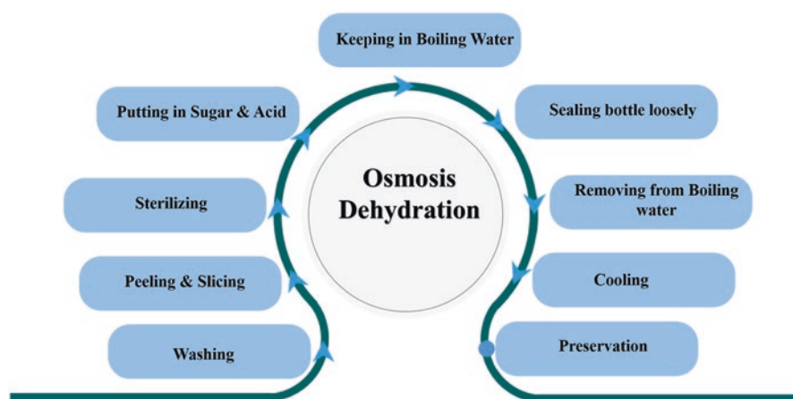
Fig. 4.28 Basic steps of osmosis dehydration of fruits and vegetables. (Adapted from Hossain et al. [79])
