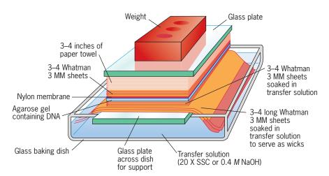
**FIGURE 14.11** Procedure used to transfer DNAs separated by gel electrophoresis to nylon membranes. The transfer solution carries the DNA from the gel to the membrane as the dry paper towels on top draw the salt solution from the reservoir through the gel to the towels. The DNA binds to the membrane on contact. The membrane with the DNA bound to it is dried and baked under vacuum to affix the DNA firmly prior to hybridization. SSC is a solution containing sodium chloride and sodium citrate.
