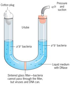
■ FIGURE 8.9 The U-tube experiment with bacteria. The U-tube is used to determine whether or not cell contact is required for recombination to occur. Bacteria of different genotypes are placed in different arms of the tube, separated by a glass filter that prevents contact between them. If recombination occurs, it cannot be due to conjugation.
