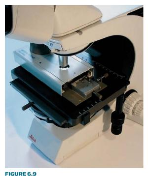
Refractive index. The heated microscope stage of the GRIM 3. The
