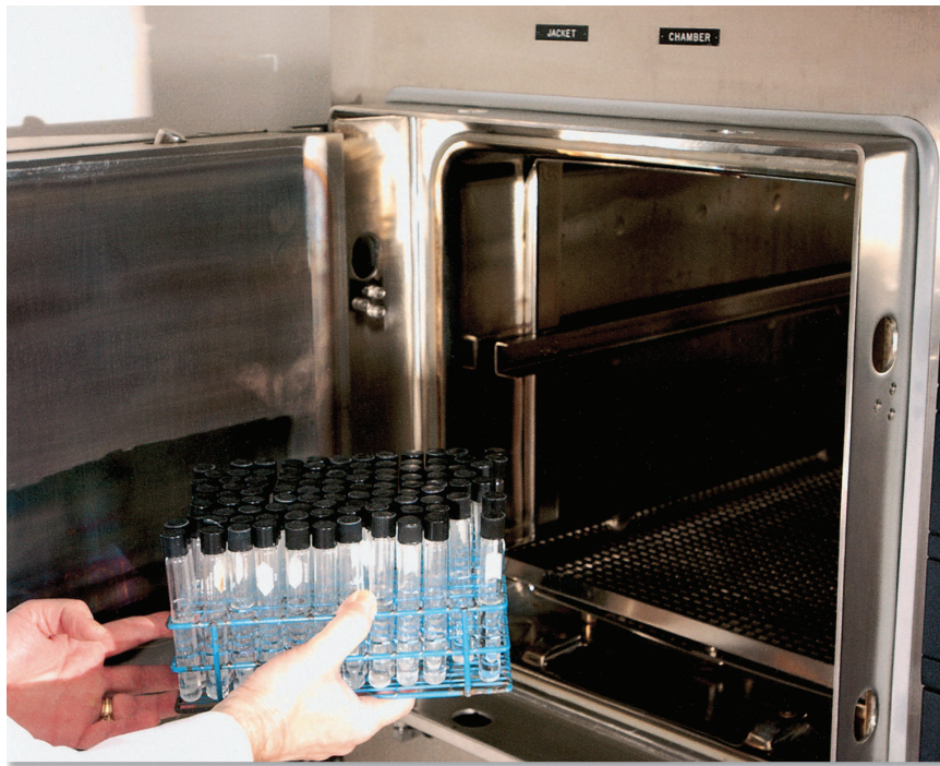
Figure 18.9 Media is sterilized in an autoclave for 15–20 minutes at 15 psi steam pressure.
