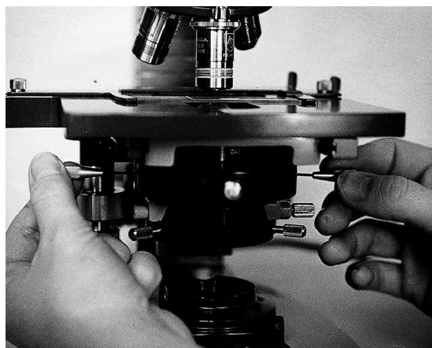
Figure 3.5 Alignment of the annulus diaphragm and phase ring is accomplished with a pair of Allen-type screwdrivers on this American Optical microscope.
