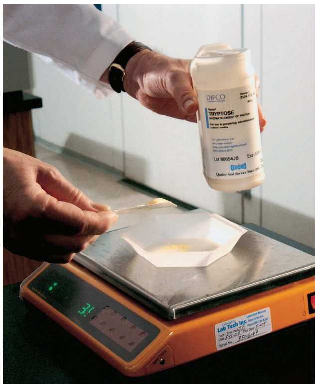
Figure 18.2 Correct amount of dehydrated medium is carefully weighed on a balance.
