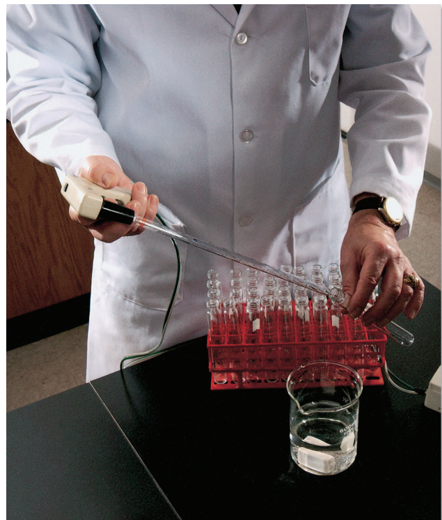
Figure 18.7 Small batches of media can be delivered with hand-held automatic pipetters.
