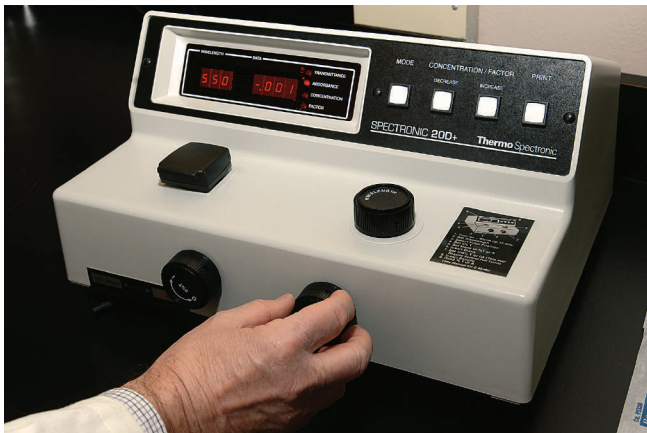
Figure 19.8 Calibration procedure for the B & L Spectronic 200 digital spectrophotometer.
