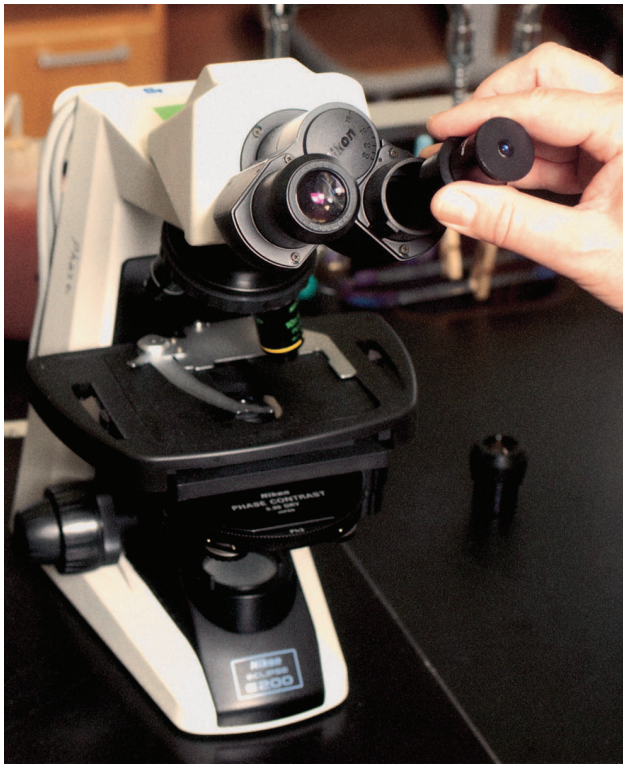
Figure 3.7 If the ocular of a phase-contrast microscope is replaced with a centering telescope, the orientation of the phase ring and annular ring can be viewed.
