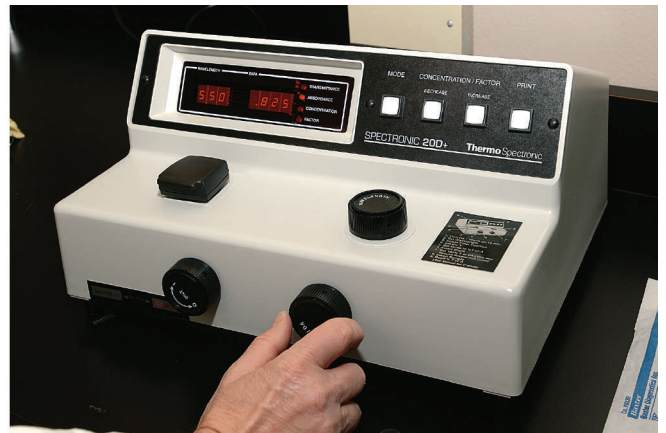
Figure 19.8 Calibration procedure for the B & L Spectronic 200 digital spectrophotometer.
