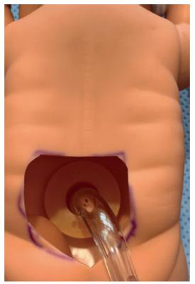
FIGURE 2.8 UAC/UVC model. Clear tubing connects silicon umbilicus to the blood bag.
