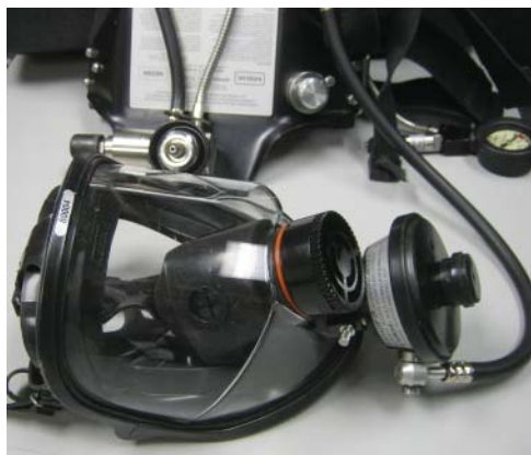
Figure 3.3 Self-contained breathing apparatus (SCBA) mask. Masks must form a tight seal to the face to provide a seal against contaminants.
