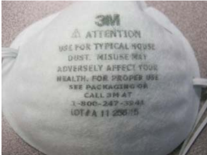
Figure 3.10 A dust mask can be worn for comfort, but it is not a respirator and does not provide sufficient protection from respiratory hazards.
