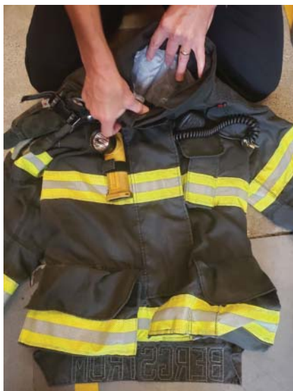
Figure 3.21 The neck of this turnout coat does not have a gauntlet. A particle blocking gauntlet would provide greater protection from contaminants.
