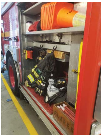
Figure 3.29 This apparatus contains a compartment for gear storage outside the cab. Storage of gear outside the cab reduces occupant exposures due to off-gassing. A more effective practice would be to bag gear at the scene and decontaminate it before reuse.
