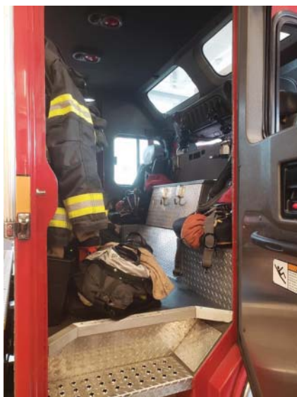
Figure 3.28 Firefighter gear is often kept inside the cab to allow easier access upon arrival at a fire scene. After the fire, gear can off-gas volatile organic compounds, and this creates another exposure source for firefighters.
