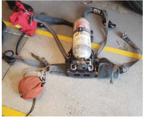
Figure 3.4 Grade D breathing air is used to provide air to an SCBA.
