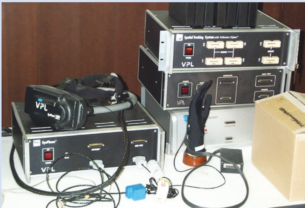
■ Fig. 1.63 An EyePhone head mounted display and a Dataglove. [Image of public domain]
