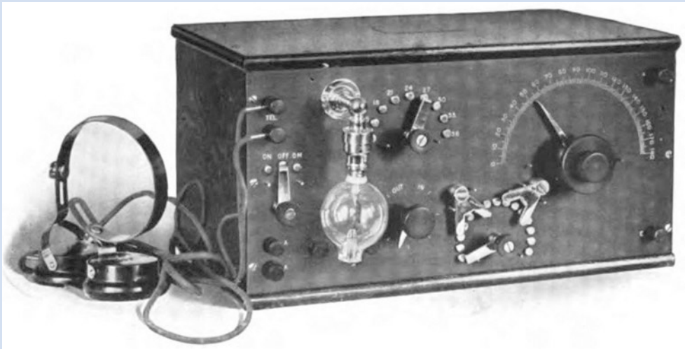
■ Fig. 1.22 A photograph of a radio receiver featuring De Forest’s Audion. [Image of public domain]
