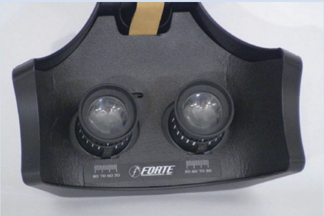
■ Fig. 1.71 The optics of the VFX1 Headgear. [Image of public domain]
