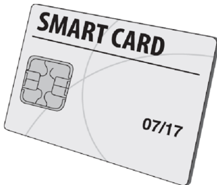
FIGURE 10.1 A smartcard's ISO 7816 interface
