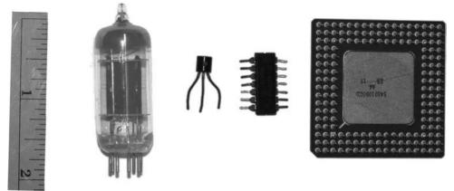
A triode, an equivalent transistor, and two integrated circuits, one SSI, containing about 25 transistors, and one VLSI, containing about 25 000 000 transistors. The scale on the left is in inches.
