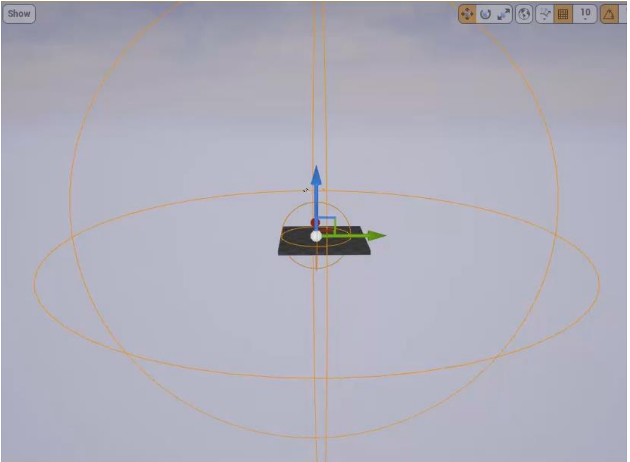
Figure 9.3.1 – The inner and outer attenuation spheres of an Ambient Sound Actor
