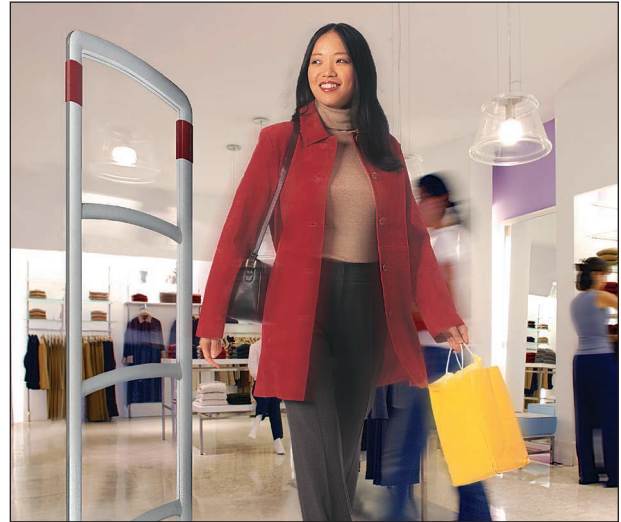
Retailers use EAS tags to reduce shoplifting. The tags contain a device that is deactivated when the merchandise is purchased. If a customer has not purchased the merchandise, an alarm is triggered when the stolen merchandise passes through sensor gates at the store's exit.
