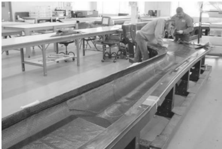
Laying up the carbon material into the tail boom tool.
