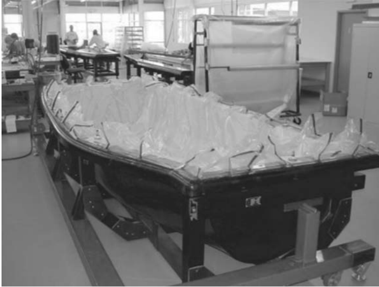
Vacuum bag on fuselage tool
