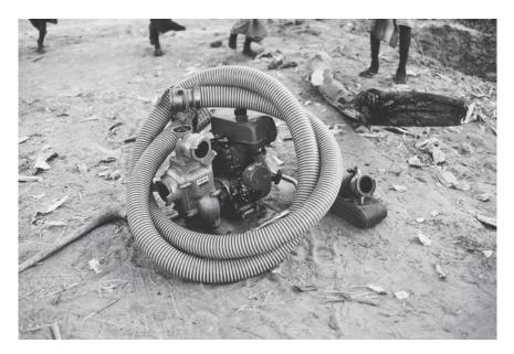
Plate 11.3 Small petrol pump, Nigeria. Small-scale irrigation using shallow groundwater and open water enabled some floodplain farmers to respond effectively to the loss of floodwaters on their land owing to upstream dams and poor rainy seasons. Photo: W. M. Adams.
