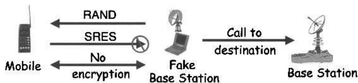
Figure 10.26: GSM Fake Base Station
