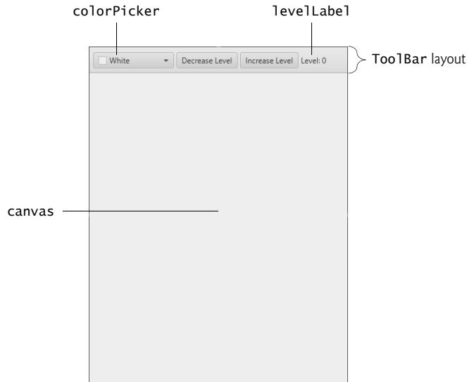
Fig. 18.18 | Fractal GUI labeled with fx:ids for the programmatically manipulated controls.
