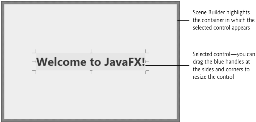
Fig. 12.4 | Welcome GUI's design after adding and configuring a Label .
