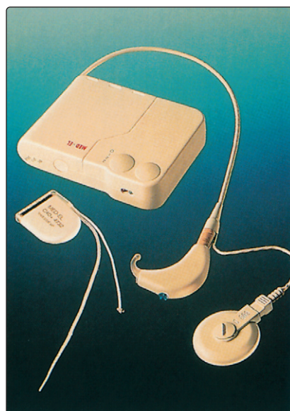
Fig. 1.24 Cochlear implantation. The device is employed to stimulate any residual cochlear nerve fibres via the electrode implanted in the scala tympani of the cochlea.
