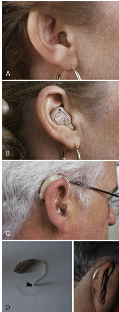
FIGURE 40-7 Common types of hearing aids. A , Completely-in-canal (CIC). B , In the ear (ITE). C , Behind the ear (BTE). D , Digital hearing aid.
