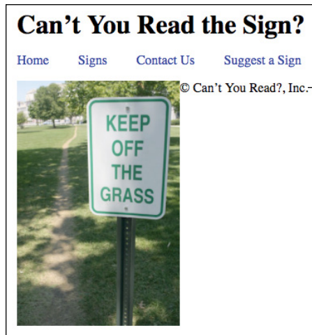
FIGURE 3-8: When the image is floated left, the footer wraps around it and ends up in a weird place.
