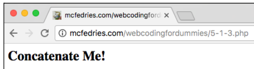
FIGURE 1-3: In PHP, you use the dot (.) operator to concatenate two strings.
