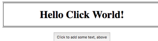
FIGURE 2-1: The click event callback function adds some HTML and text to the div element.
