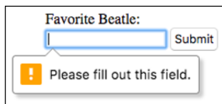
FIGURE 3-1: Add the required attribute to a form field to ensure it gets filled in.
