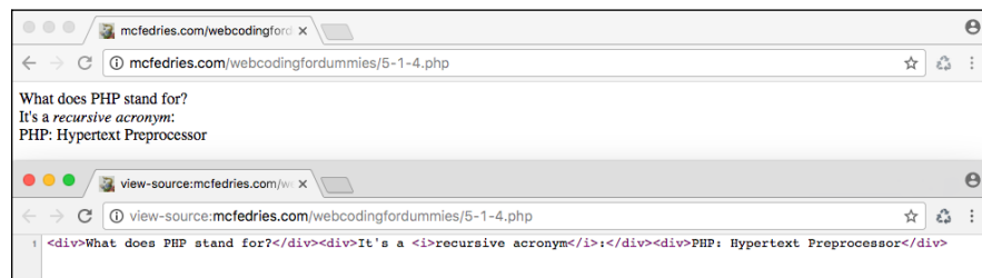
FIGURE 1-4: When you output tags and text using PHP, the strings run together in a single line in the web page source code.
