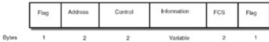
Figure 27.5: LAPD frame format.
