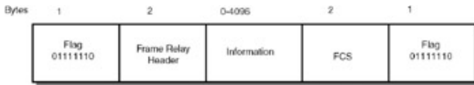
Figure 28.2: LAPF frame format.
