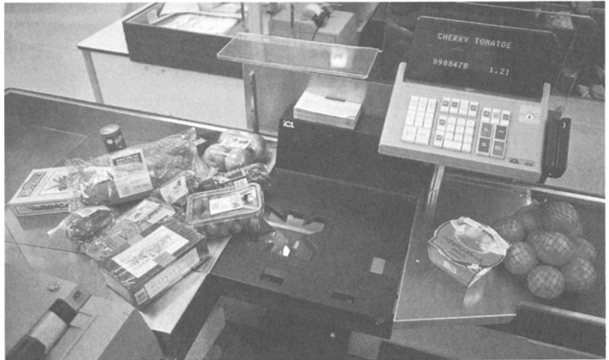
A bar code reader incorporating a light-sensitive cell, built into a shop checkout
