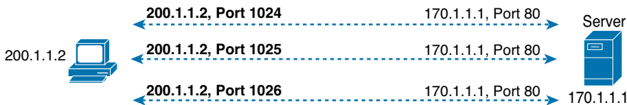
Figure 24-7 Three TCP Connections from One PC
