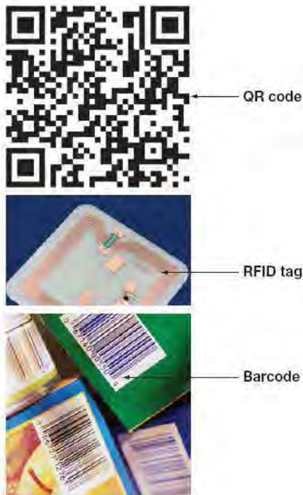
FIGURE 8.6 Barcodes, RFID tags, and QR codes.
